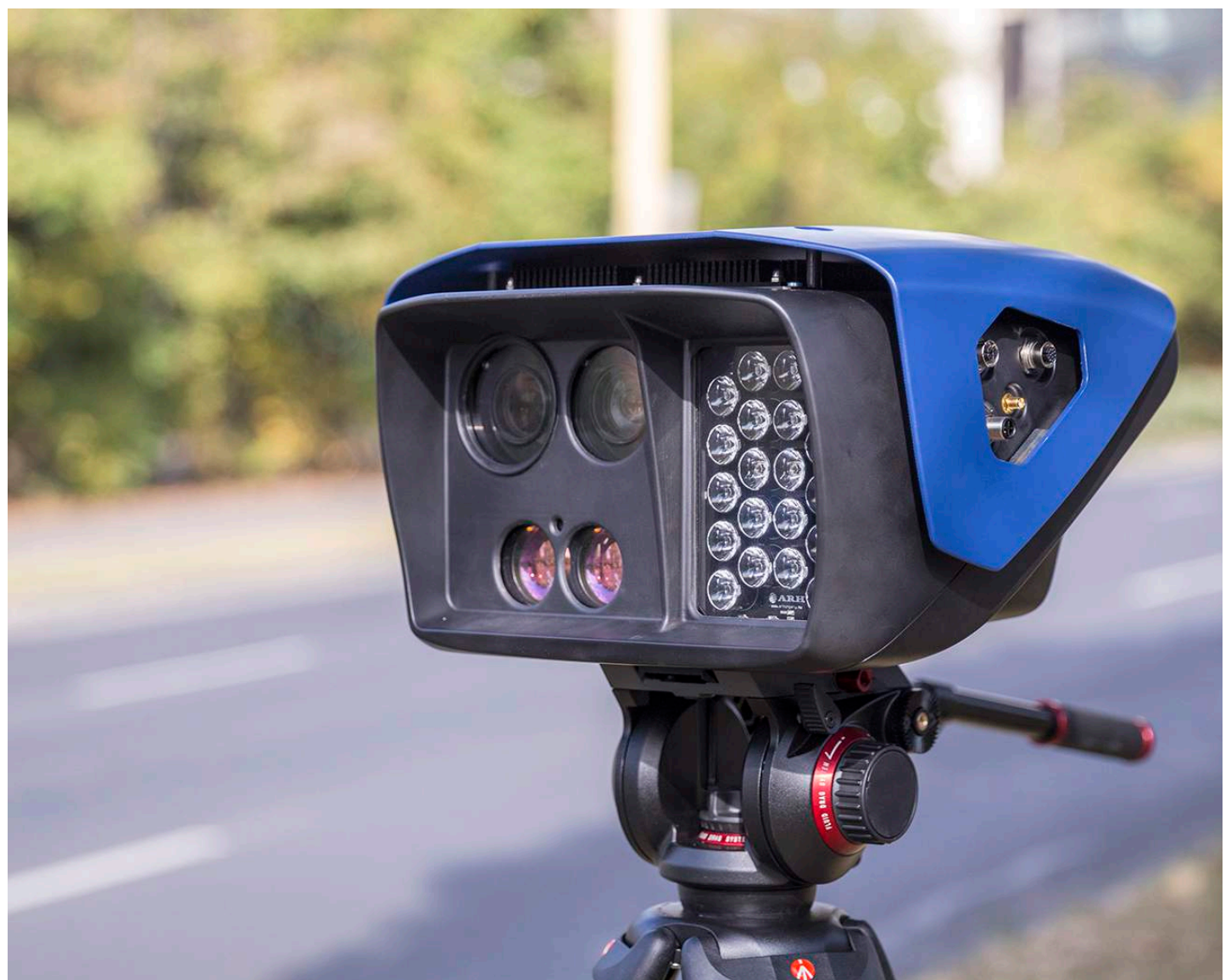
Portable traffic enforcement system used by the Hungarian police. The rows of infrared LEDs are visible on the right. //Wikipedia
