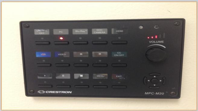
Please take a moment and locate this Crestron wall panel control by the teacher's station. Pressing an input will start up the system. For example, pressing the PC button is equivalent to turning ON the system. Be advised that the system takes 1 to 2 minutes to power on. Please be patient.
