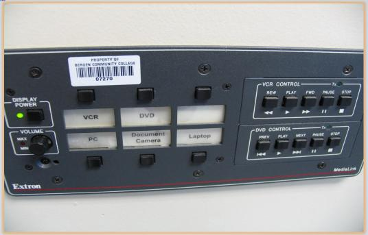
Please take a moment and locate this control panel on the wall by the teacher's station. Once located, press the Display Power button for 4 seconds then let go. The green light will blink indicating that the system is powering on. Be advised that it may take 1 to 2 minutes for the system to fully turn on. Please be patient.
