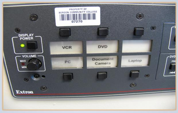
When finished, please power off the system by pressing the Display Power button for a good 4 seconds, let go and the light will start blinking again. This indicates that the system is powering off and cooling down.
