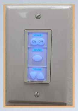
You are now ready to choose what equipment image you would like projected. Press the "SOURCE" button to select an input, you may have to give the system a couple seconds to adjust between sources.
